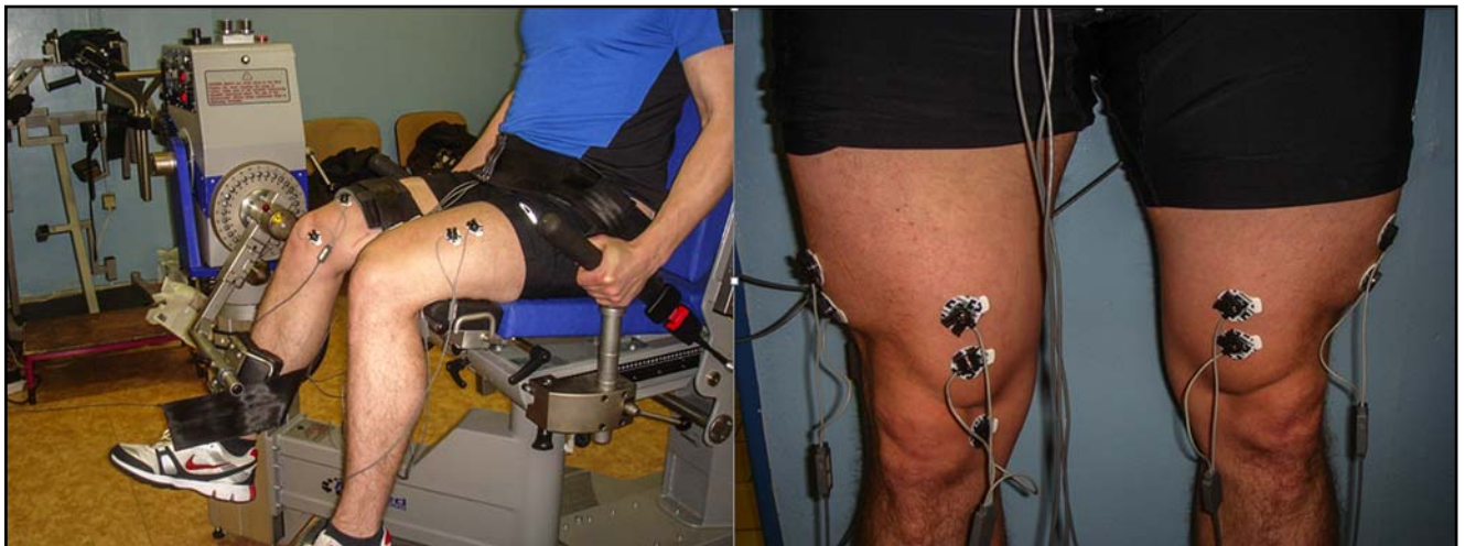
Fig. 1. Body position during maximum voluntary isometric test (MVIC) and quadriceps electrodes placement.
